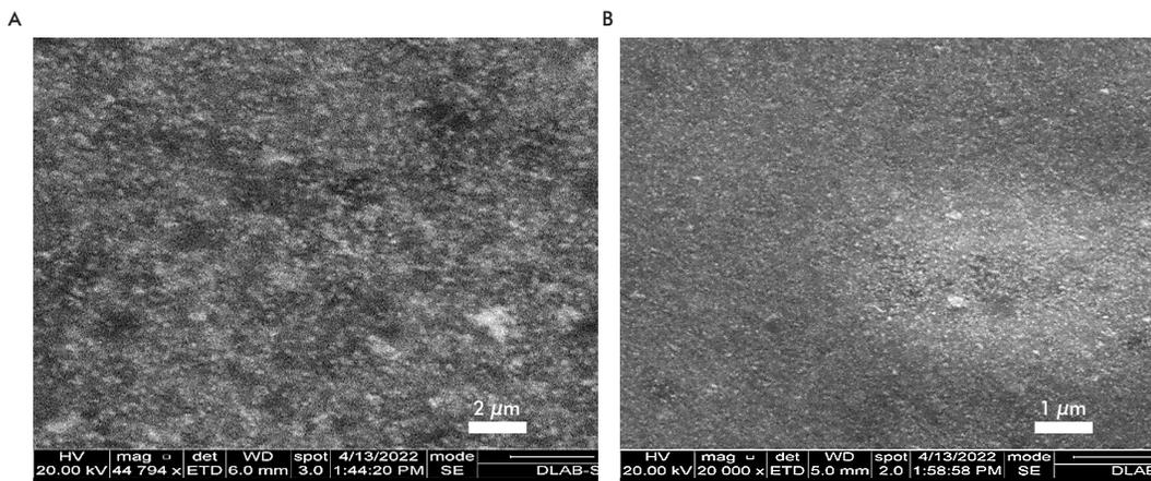
Figure 5. Scanning electron microscopy images of silver nanoparticles (AgNPs) prepared biosynthesized from plant leaf extracts. A) Olive AgNPs. B) Eucalyptus AgNPs.
