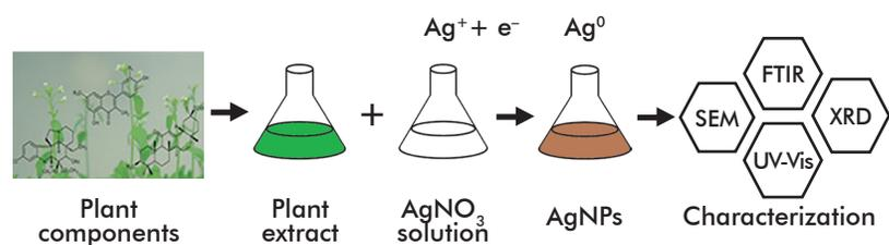
Figure 1. Diagram of the synthesis process and characterization of silver nanoparticles (AgNPs) by reduction of  $\text{Ag}^+$  into  $\text{Ag}^0$ . AgNPs: Ag nanoparticles. SEM: scanning electron microscopy. FTIR: Fourier transform infrared spectroscopy. XRD: X ray diffraction. UV-vis: ultraviolet-visible spectrometry.
