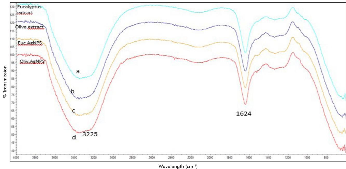
Figure 4. Fourier Transform Infrared spectroscopy (FTIR) analysis of olive and eucalyptus leaf extracts and derived biosynthesized silver nanoparticles (AgNPs).
