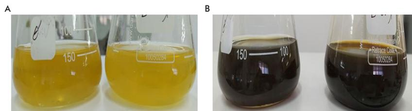
**Figure 2. Color change of plant extract solution 24 h after adding it to a silver solution. A) Olive extract solution. B) Eucalyptus extract solution.**
